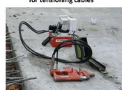
Hydraulic jack machine for tensioning cables
