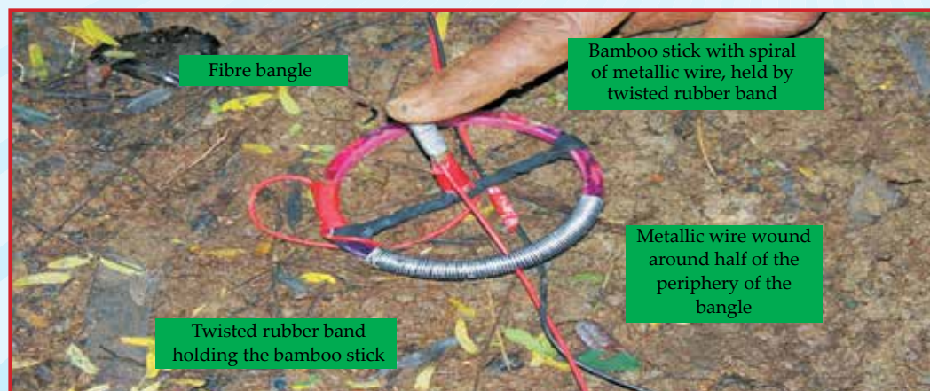
Fibre bangle, rubber band, bamboo stick used in anti handling mechanism
