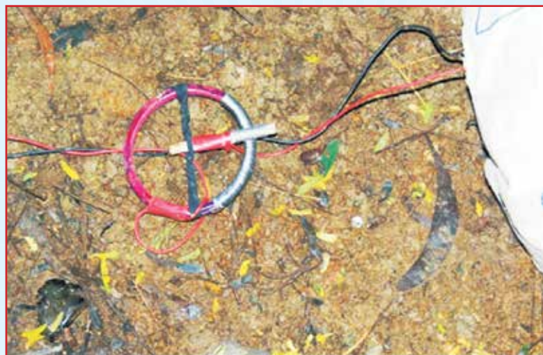
Fig-1: Bag placed on bangle which separated bamboo stick and metallic wire over bangle. Fig-2: Displaced bag which brought bamboo stick in contact with metallic wire over the bangle
